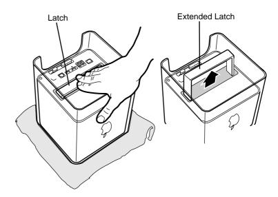
Allow the latch to extend completely.
